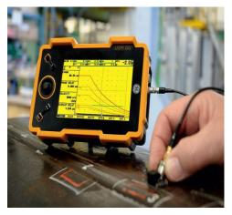
Phased Array Ultrasonic testing
